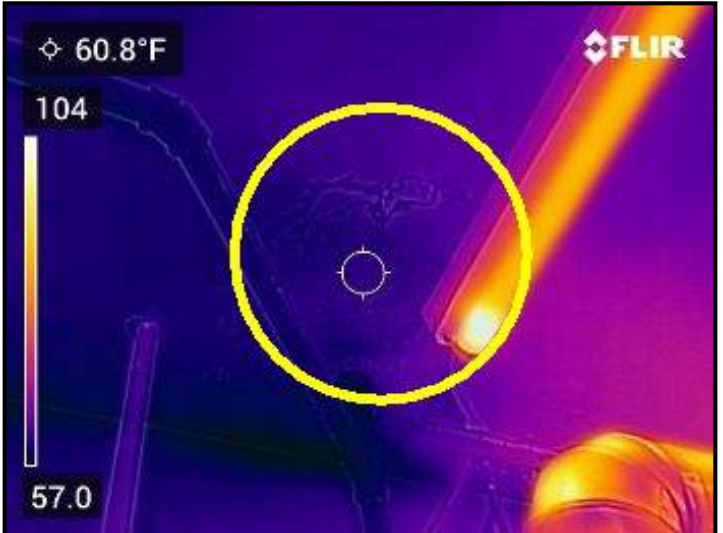
No current moisture observed around water piping above boiler
